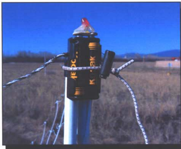
Figure 5—LEDs (light-emitting diodes) attached to two sides of a portable electric mesh fence can warn campers or animals before they touch or run into the fence.
