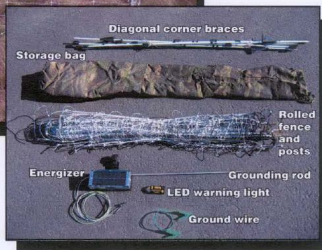
Figure 1—This portable electric mesh fence system is a potential alternative for storing food, garbage, and other attractants in bear country.
